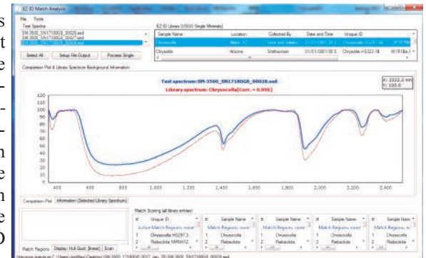
A spectra of a chrysocolla sample from a copper mine in Canada with a known sample from the USGS library.
