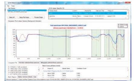
EZ-ID identifying calcite using match regions to focus on specific absorption features.
