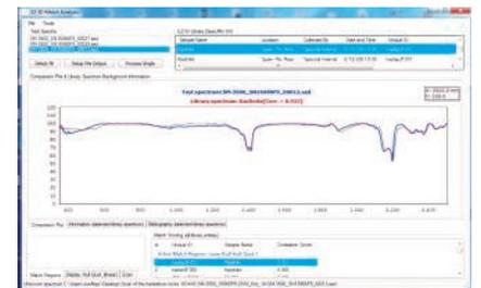
EZ-ID identifying sample of kaolinite, a clay sometimes found with dolomite and calcite.
