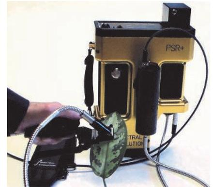
*The PSR+ with our unique leaf clip with a built-in white reference and a separate tungsten halogen illumination source to keep heat away from the sample during measurement.*
