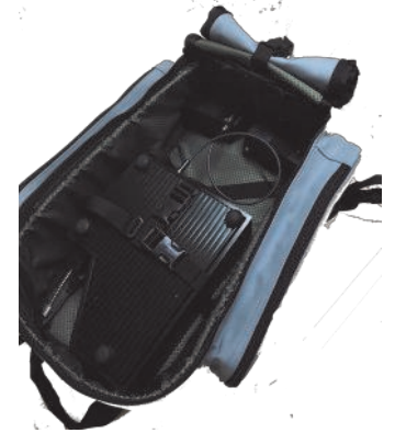
The oreXpress is a field spectrometer designed to provide high resolution/high sensitivity collection of mineral spectra in situ. When used with EZ-ID mineral identification software it offers a mineral analyzer that can be used at outcrops or trenches or logging core in a core shack.
