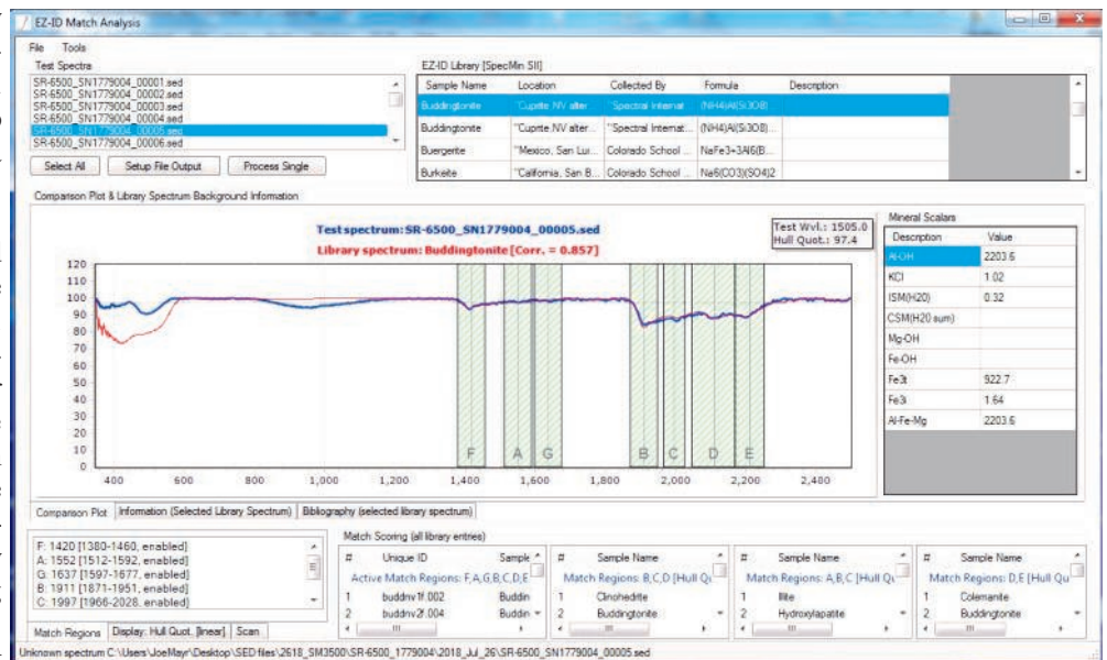
EZ-ID provides over 2600 spectra for more than 1000 minerals. Above is a sample spectra matched to a buddingtonite sample in the SpecMIN library.
