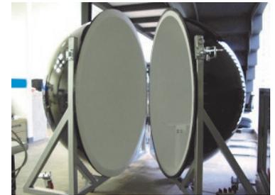
*Detailed calibrations using integrating spheres are used to fully characterize satellite instruments.*
