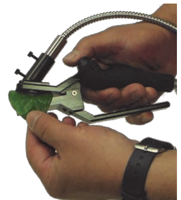
An optional leaf clip includes an internal reference standard.
