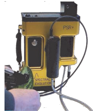
A field portable spectroradiometer provides valuable information for forest canopy research.
