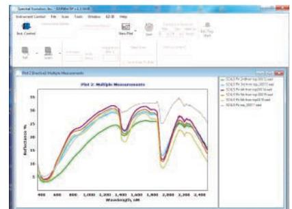
*DARWin SP Data Acquisition software is included with every SPECTRAL EVOLUTION spectroradiometer. The software allows you to display multiple scans of different soil samples for comparison.*
