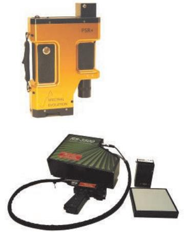
*Soil analysis using NIR spectroradiometers like the PSR+ and RS-3500 can measure total carbon (TC), water, carbon, nitrogen, clay, and pH.*
