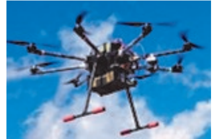
SPECTRAL EVOLUTION PSR+ mounted to an eight rotor UAV.
