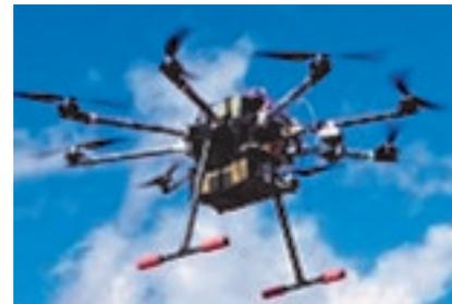
*SPECTRAL EVOLUTION PSR+ mounted to an eight rotor UAV.*
