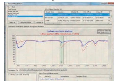
Smectite/montmorillonite sample identified with EZ-ID
