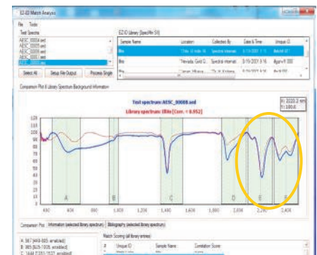
Illite sample—sometimes illite and smectite spectra look very similar. Here you clearly see the difference with a doublet absorption feature for illite between 2300-2500nm.
