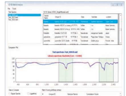
Kaolinite spectra matched by EZ-ID to a known sample of the clay in the SPECMin library
