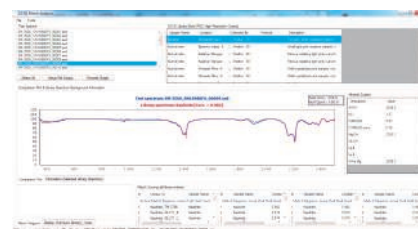
EZ-ID software identifies minerals in real-time by matching your target spectra against a known spectral library such as the USGS library, the SpecMIN library or the GeoSPEC library.
