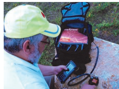
oreXpress, oreXplorer and oreXpert spectrometers are ideal for single-user field mining exploration.
