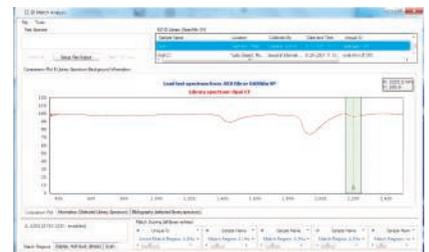
*EZ-ID software identifies minerals in real-time by matching your target spectra against two known spectral libraries. Above is a sample of an Opal-CT scan in the library showing the 1400 and 1900 nm water features as well as the Si-OH vibrational feature at 2250nm.*
