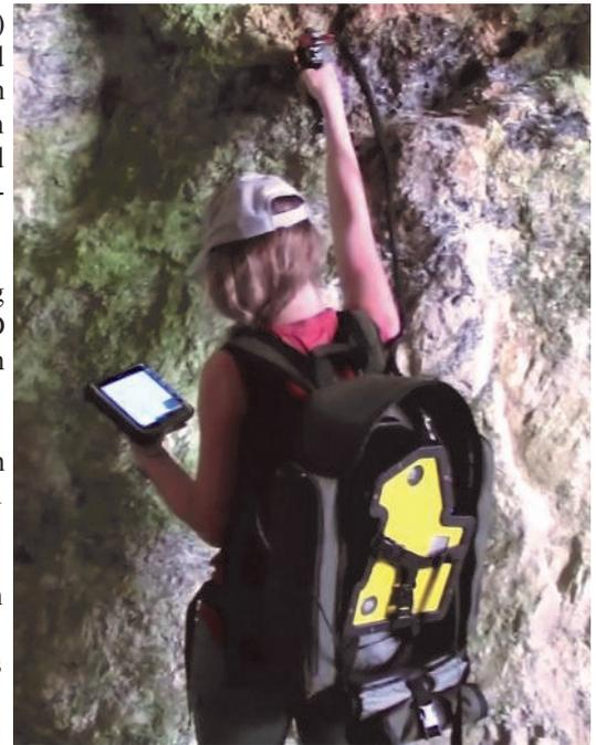
**SPECTRAL EVOLUTION field spectrometers include the oreXpress, oreXplorer and oreXpert. They are carried in a backpack for field use and work with an optional ALGIZ 8X tablet.**
