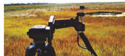
*Measuring diffuse solar irradiance with a diffuser.*
