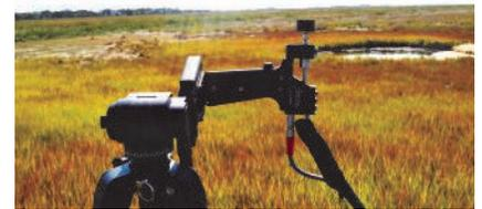
*Measuring global solar irradiance with a diffuser.*
