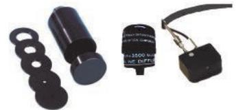
*Gershun tube, in-line diffuser and right-angle diffuser.*
