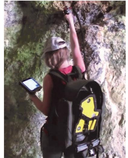
*The oreXpress, oreXplorer and oreXpert are rugged field spectrometers for identifying minerals in situ.*
