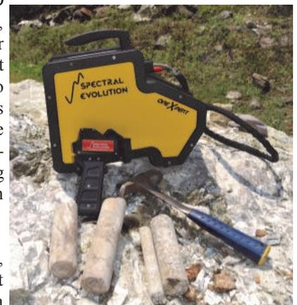
*oreXpert has the highest resolution in a field portable spectrometer for mineral identification.*
