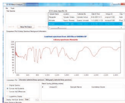
This EZ-ID display shows a SpecMIN library sample of monazite which may also contain HREEs.
