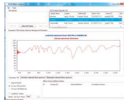
EZ-ID software provides mineral identification. Here is a sample of xenotime from the SpecMIN library.
