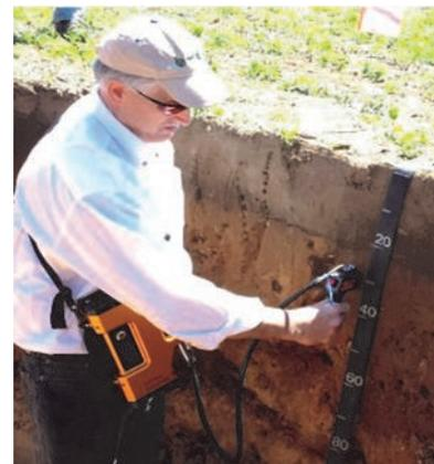
*SPECTRAL EVOLUTION field spectrometers include the SR-6500, RS-5400, RS-8800, PSR+ and RS-3500. Here a researcher is using the PSR+ and a contact probe for soil measurements in a pit.*
