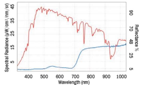
**Reflectance scan and scan of grass in DARWin SP Data Acquisition software multiplot window.**
