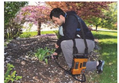
Our spectroradiometers are designed for field use: rugged, lightweight, battery operated. Our unique leaf clip includes an integrated light source and built-in reflectance standard for ease-of-use and keeps your sample away from heat.
