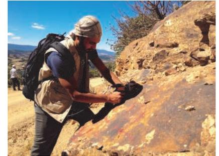
*oreXpress spectrometers are used to better understand and map mineral alteration zones in the field.*
