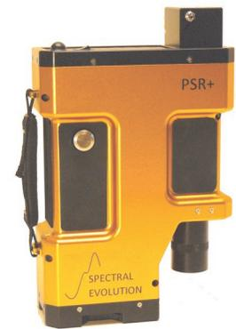
*The PSR+ field spectroradiometer is ideal for measuring LED chromaticity and luminosity to meet FAA requirements.*
