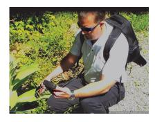
SPECTRAL EVOLUTION's spectroradiometers and spectrometers are ideal for measuring and analyzing vegetation stress as an indication of hydrocarbon leakage.
