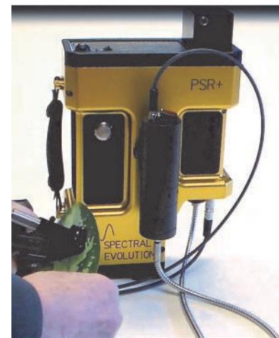
PSR+ has a spectral range from 350-2500nm and features auto-dark correction, auto-exposure, and auto-shutter for one-touch operation.
