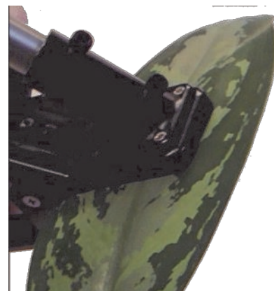
Take leaf reflectance measurements in the field with the PSR+ and our leaf clip attachment.
