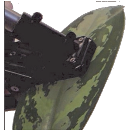
Take leaf reflectance measurements in the field with the PSR+ and our leaf clip attachment.
