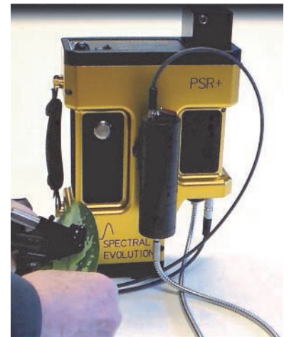
PSR+ has a spectral range from 350-2500nm and features auto-dark correction, auto-exposure, and auto-shutter for one-touch operation.
