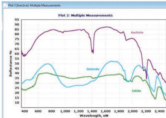
In a multi-spectral plot, the kaolinite clay in this limestone mixture can be differentiated by the doublets near 1400nm and 2200 nm. While dolomite and calcite have similar absorption features, there are subtle differences. Dolomite has features at 1858, 1978, and 2320 nm; calcite at 1875, 1995, and 2330nm.
