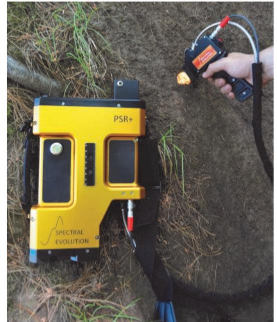
*The PSR+ is a rugged NIR field spectroradiometer that can be used for soil analysis with a contact probe, benchtop probe with compactor or pistol grip with FOV lens.*
