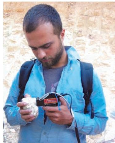
*oreXpress spectrometers are used to better understand and map mineral alteration zones quickly and accurately.*
