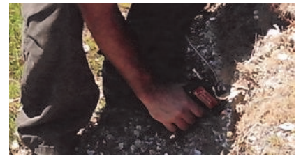
Soil analysis using NIR spectroscopy can measure water, carbon, nitrogen, clay, pH, and organic matter.
