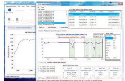
*EZ-ID screen with a scan of kaolinite. Kaolinite is a soft mineral that affects ore processing. It has been identified here using the USGS library.*
