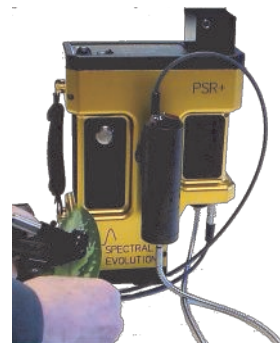
The PSR+ with our unique leaf clip can take field measurements to determine plant health.
