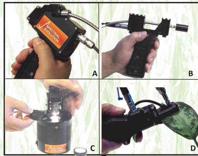
The PSR+ can also be used with fiber mount options and a range of accessories including (A) ergonomic sample contact probe with a built-in 5W halogen light source; (B) pistol grip with 1,2,3,4,5, 8 and 10° fiber mount lenses; (C) benchtop probe with sample tray and compactor; and (D) a custom leaf clip with a pushbutton trigger and an integrated light source. An integral swing-away reflectance panel provides easy reference measurements.
