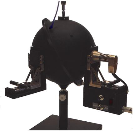
*RT Sphere can measure reflectance, transmittance, and absorption.*
