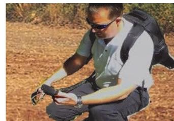
**Soil analysis using NIR spectroscopy can measure phosphorus, water, carbon, nitrogen, clay, pH, and organic matter.**
