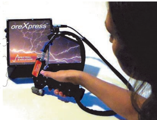
The oreXpress can use a 3mm or 10mm contact probe or a benchtop probe with compactor for chips and powder samples.
