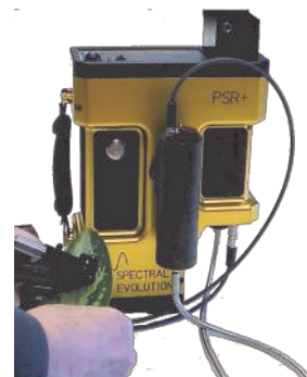
PSR+ with uniquely designed leaf clip for vegetation measurements
