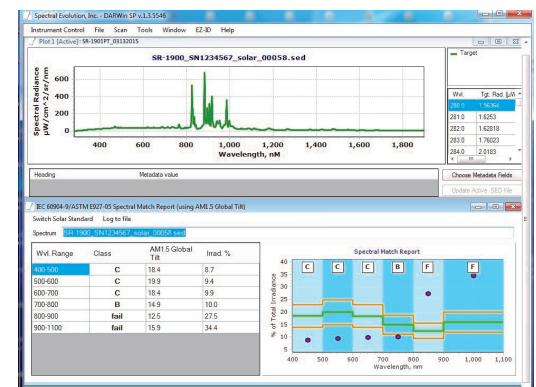
A spectral match report from the SR-1901PT showing the classification of a low cost solar simulator.
