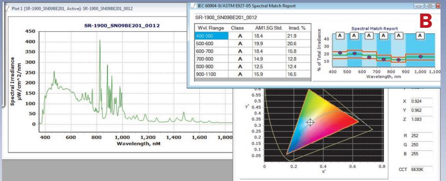
The full range SR-3500 was used to measure outdoor solar radiance reflected off a white reflectance plate, using a 4° lens foreoptic. Pull down menus allow for easy calculation of integrated energy measurement. All SPECTRAL EVOLUTION Spectroradiometers are lightweight and easy to carry anywhere.
