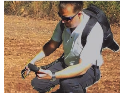
The PSR+ can be used to measure the salinity of soil in semi-arid and arid environments.
