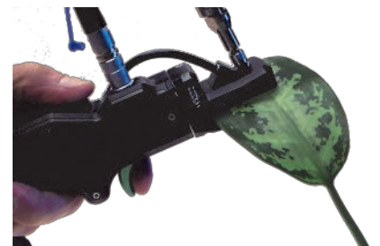
The leaf clip includes a tungsten halogen light source and internal reference standard for ease-of-use and accurate measurement without affecting the sample.
