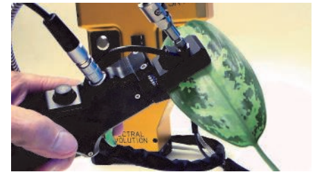
Take leaf reflectance measurements in the field with the PSR+ or RS-3500 bundle and our optional leaf clip.
