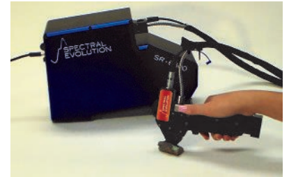
The SR-6500 delivers high resolution/high sensitivity for field identification of minerals.
