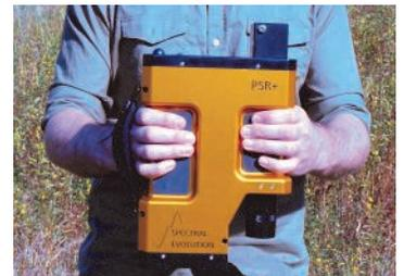
*The PSR+ and all our spectroradiometers are designed for reliability in the field with no moving optical parts to breakdown.*
