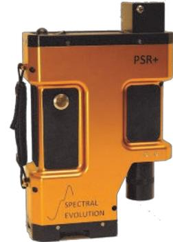
*The PSR+ , our most popular field spectroradiometer, uses one 512 element silicon photodiode array and two InGaAs extended photodiode arrays to cover the full 350-2500nm spectral range with the highest resolution and sensitivity in a field handheld spectroradiometer.*
