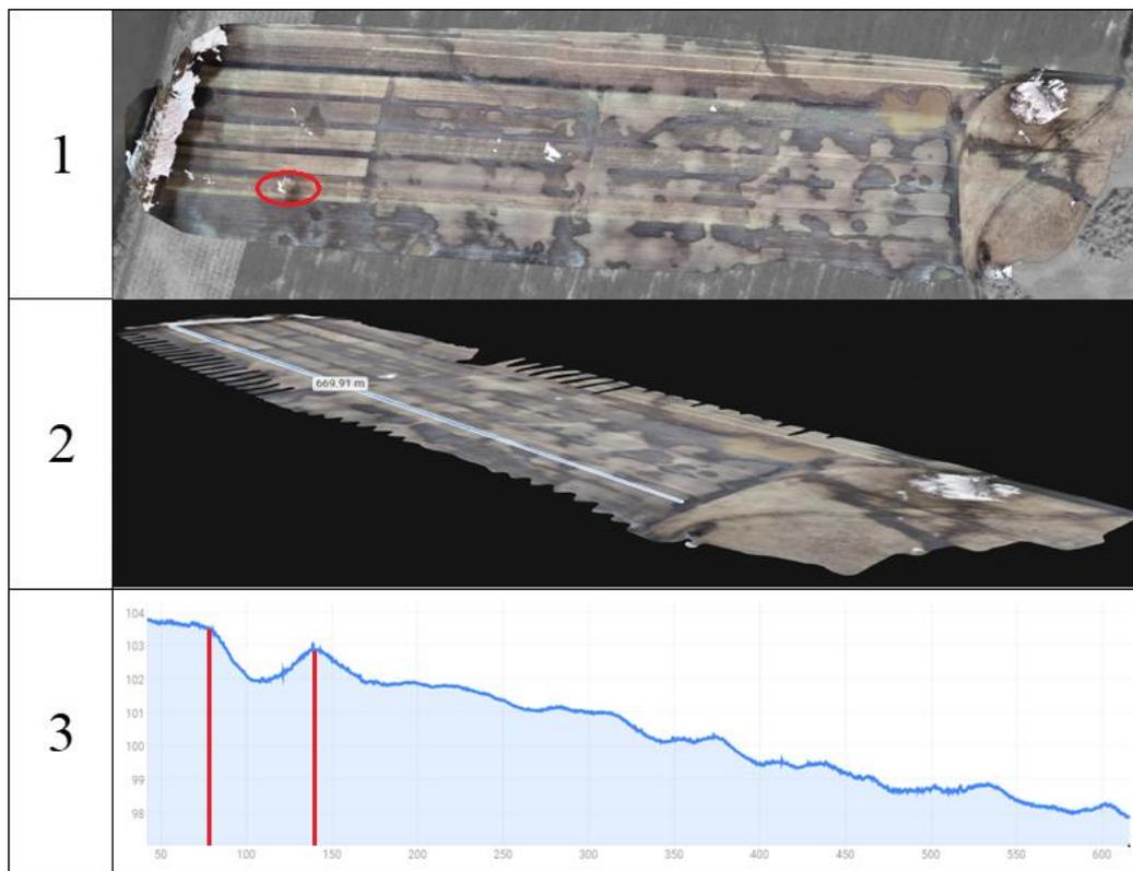
**Figure 1.** Processed survey results. 1 - orthophoto mosaic, 2 - 3D model, 3 - vertical profile for strip No 5. The red circle and lines mark the area with a 1 m decrease in height.
