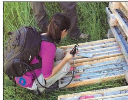
*oreXpress, oreXplorer and oreXpert spectrometers are ideal for core logging applications.*
