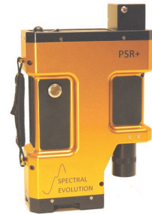
A field portable spectroradiometer can be used for a wide range of vegetative studies in the field
