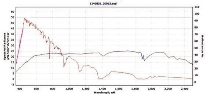
*Blue line is surface scan taken with a SPECTRAL EVOLUTION field spectrometer. The red line represents the solar radiance of the reflected light.*
