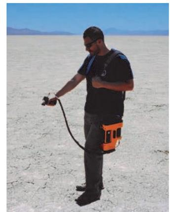
*Vicarious radiometric calibration can be done with a PSR+ spectroradiometer.*
