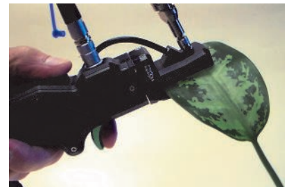
An optional leaf clip includes an internal reference standard and an external trigger
